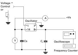
$\rm C_L$  = Load 15pF (HCMOS or 10k $\Omega$  // 10pF (Clipped Sinewave), inclusive of probe and jig capacitance.  $\rm CS$  = 100nF
